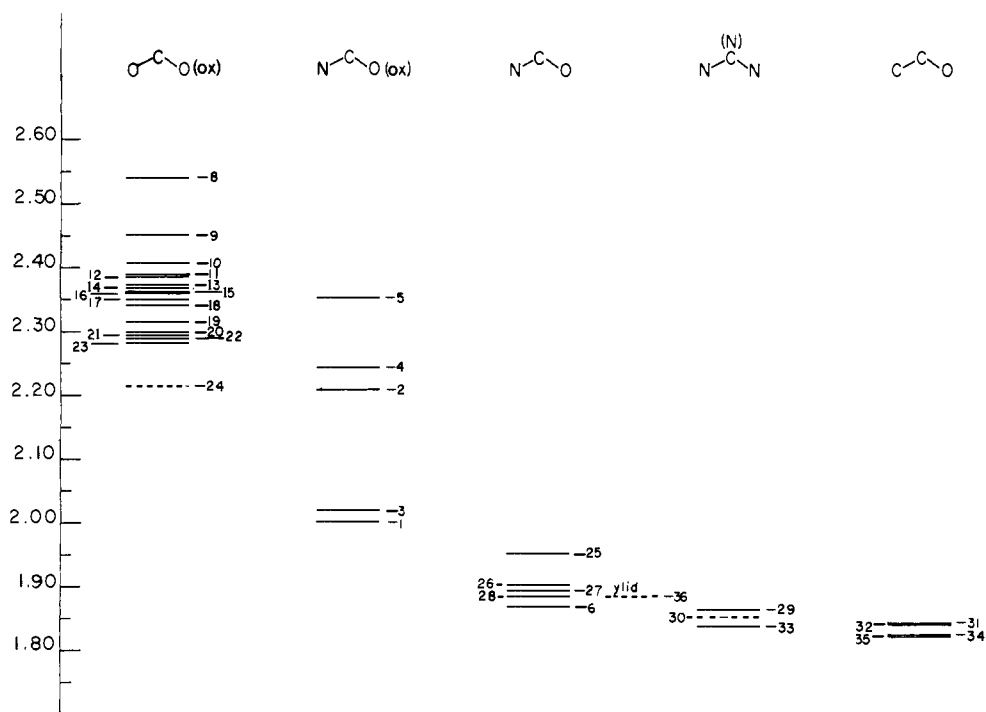
Figure 6. A plot of Cr-Cr quadruple bond distances (ordinate) for various types of bridging bidentate ligands. (ax) in columns 1 and 2 indicate that axial ligands are present. Compound numbers correspond to those in Table VIII.
